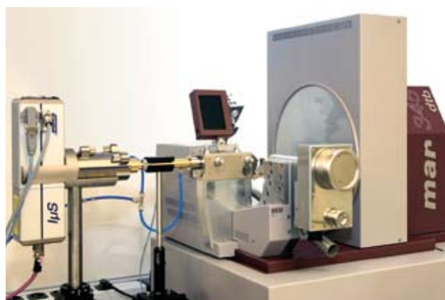
Fig. 1: Incoatec Microfocus Source I \mu S™ in combination with a marresearch desktop beamline® and an imaging plate detector mar345.
