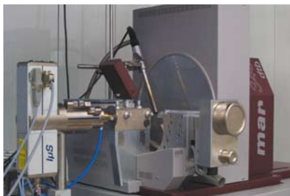
Fig. 2: Incoatec Microfocus Source I\mu S^{\text{TM}} combined with a mardtb and imaging plate detector mar345. The hot-air blower is pointed to the sample.
