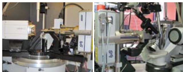
Fig. 1: The Incoatec Microfocus Source I \mu S in combination with a Bruker Smart Apex II (left) and a Nonius Kappa CCD diffractometer (right).
