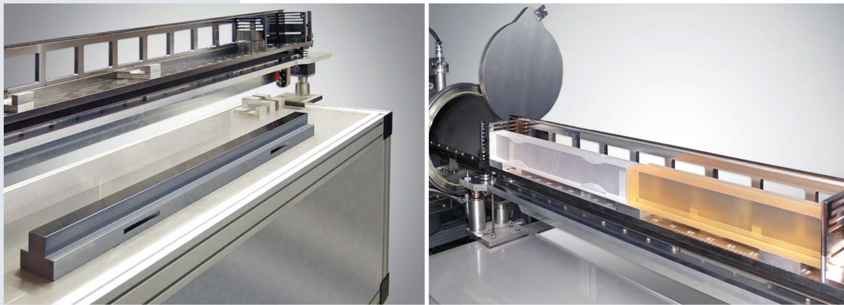
100 cm Si mirror with special carbon coating (left) and 2 substrates -110cm- on the carriage (right).
