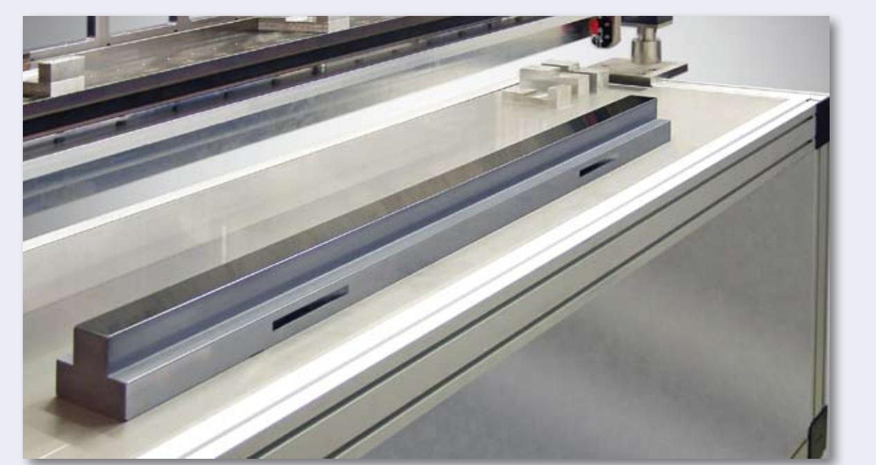
Total reflection optics are used for beam guidance and alignment. The length often exceeds 100 cm due to small incidence angles.
