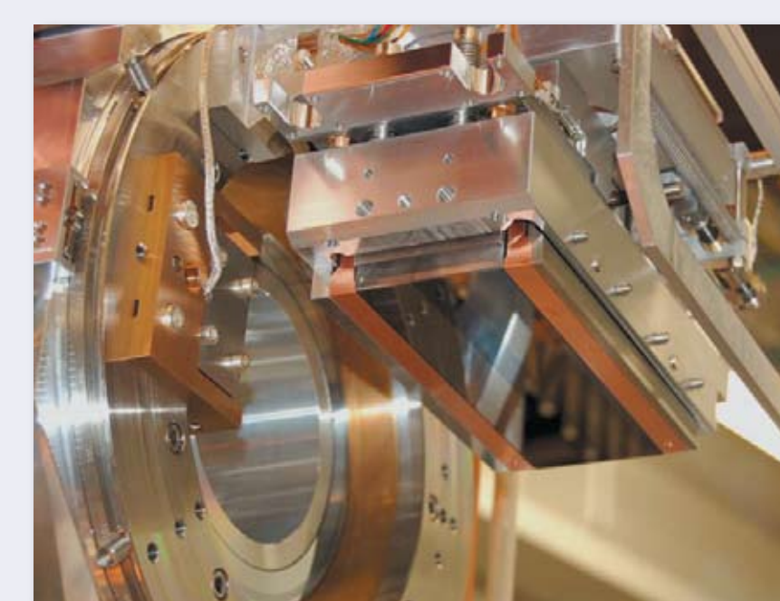
Three-stripe multilayer optics for tomographic microscopy and coherent radiology. The coatings are optimized for different beam energies (TOMCAT at SLS). (M. Stamparoni, PSI)
