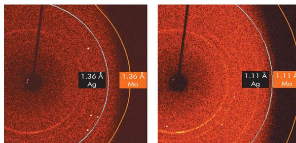
Figure 4: Diffraction patterns illustrating the gain in resolution with Ag radiation ( $2\theta = -15^\circ$ ,  $\omega = -160.1^\circ$  (left) resp.  $-162.2^\circ$  (right))
