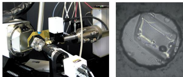
Figure 1: The Ag- $l\mu S$  on a Bruker AXS APEX II QUAZAR goniometer with a Be-free DAC and modified collimator (left); gabapentin crystal (F. P. A. Fabbiani et al., *CrystEngComm*. 2010, 12, 2354) in a 0.3 mm inconel gasket, 0.8 GPa (right).
