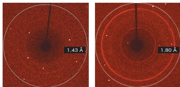
Figure 3: Diffraction patterns of the gabapentin heptahydrate crystal ( $C_9H_{17}NO_2 \cdot 7H_2O$ ;  $\varnothing \approx 0.25$  mm) grown in-situ in a Be-free DAC ( $2\theta = 0^\circ$ ,  $\omega = 0.5^\circ$  (Ag) resp.  $4^\circ$  (Mo),  $\varphi = 0^\circ$ ): Ag- $\mu$ S (left), Mo sealed tube (right). Please note that the crystal moved slightly during data collection and, therefore, the two diffraction patterns do not show the same Bragg peaks.
