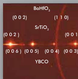
Measurement of textured \text{BaHfO}_3 nanoparticles deposited on YBCO with Cu- \mu S on a Bruker GADDS system
