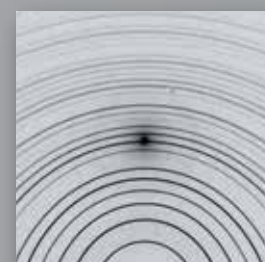
Diffraction pattern of \text{LaB}_6 measured with Mo- \mu S and a Mar imaging plate detector
