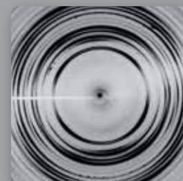
Diffraction pattern of a \text{CaCO}_3 -cuttlebone measured with Mo- \mu S and imaging plate detector
