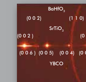
Measurement of textured BaHfO_3 nanoparticles deposited on YBCO with a Cu- \mu S on a Bruker GADDS system
