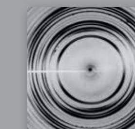
Diffraction pattern of a CaCO_3 -cuttlebone measured with Mo- \mu S and imaging plate detector
