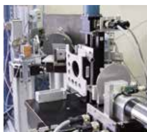
XRD/XRR setup in synchrotron optics lab at ESRF in Grenoble, France
