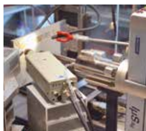
Combined XRF/XRD setup for painting analysis in Antwerp, Belgium
