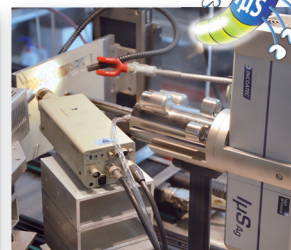
Combined XRF/XRD setup for analysing paintings in Antwerp, Belgium
