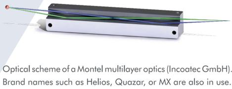
Optical scheme of a Montel multilayer optics (Incoatec GmbH). Brand names such as Helios, Quazar, or MX are also in use.
