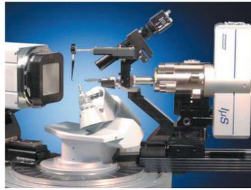
Sealed tube microfocus source  $\mu\text{S}$  (Incoatec GmbH, Cu anode, 50  $\mu\text{m}$  focal spot, 30 W), equipped with a Quazar multilayer optics.
