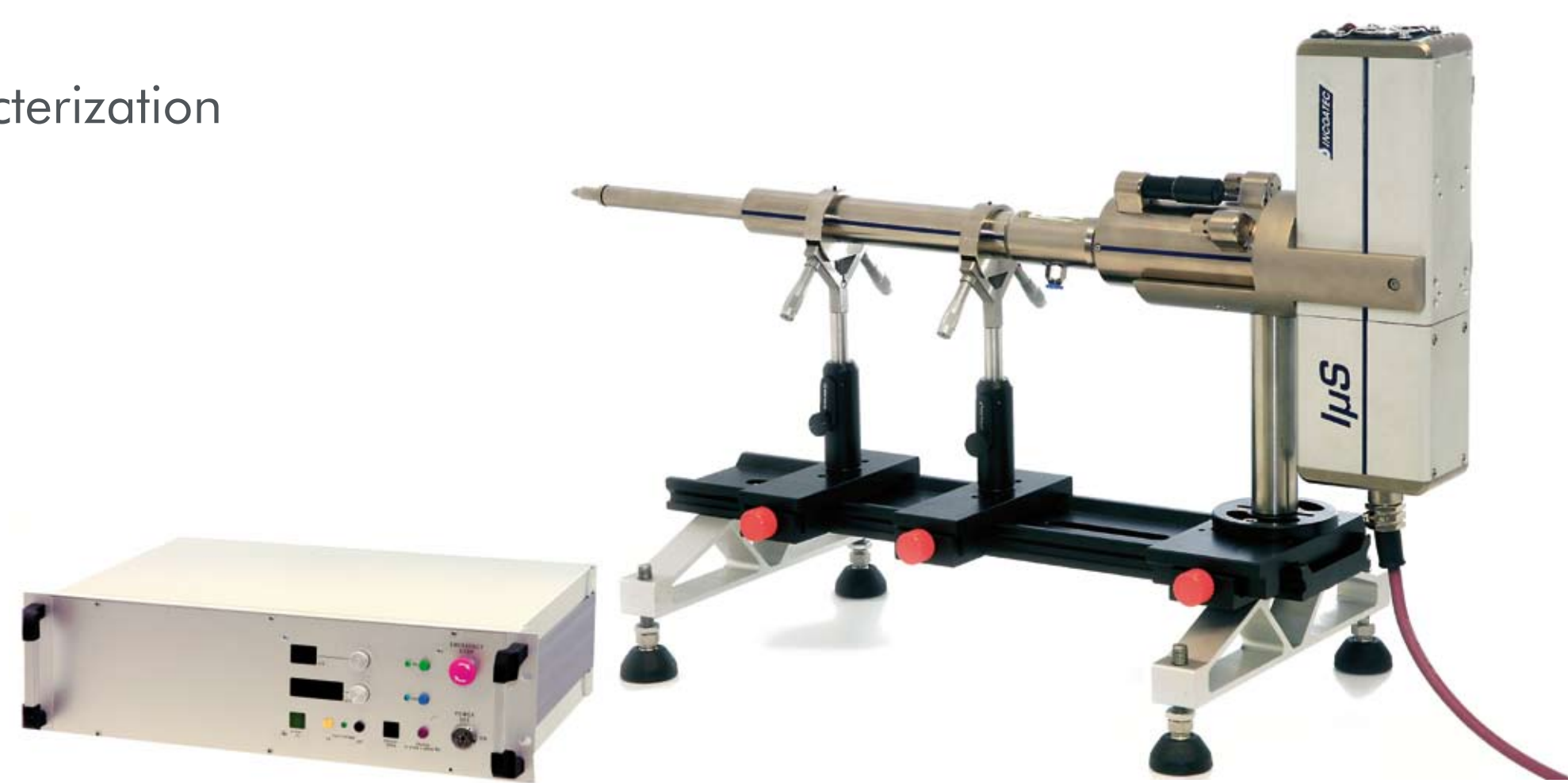
\mu S System with optics housing and 19" wide generator
