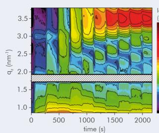
Time resolved evolution GISAXS reciprocal space map of the 10x W/B<sub>4</sub>C multilayer mirror with visible Bragg peak and Kiessig fringes
