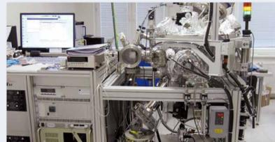
The Dual Ion-beam sputtering unit in Bratislava was upgraded with an in-situ GISAXS set-up. As a source an  $\mu\text{S}$  with a special collimating optics for SAXS is mounted on a Hexapod. Together with the 2-dim detector Dectris Pilatus 200K dynamic measurements during thin film growth become feasible.
