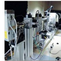
$\mu\text{S}$  + SCATEX upgrade on a customized SAXS setup in Hamburg
