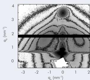
Reciprocal space map of 10 periods W/B<sub>4</sub>C multilayer mirror with 1.5 nm period thickness measured ex-situ by GISAXS in deposition chamber
