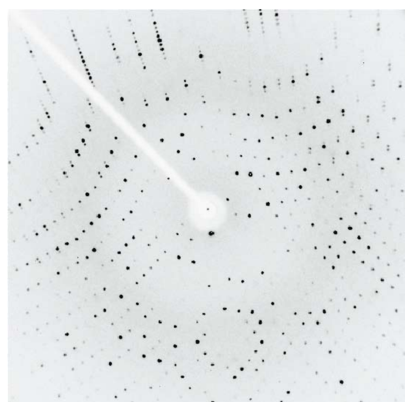
Fig. 2: Statistical data and a typical diffraction pattern of thaumatIN ( a = b = 57.86 Å; c = 149.55 Å; P4_12_2 ; T = 100 K; 208 amino acids / ASU). All 17 S atoms have been found in the initial phasing with SHELXD. (* values for outer resolution shell 1.52 – 1.42 Å).
