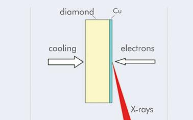
Principle of the diamond hybrid anode used in the air-cooled IµS DIAMOND.
