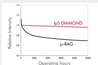
Comparison of the decay in the relative intensity over time for a low power microfocus rotating anode and for an IµS DIAMOND.
