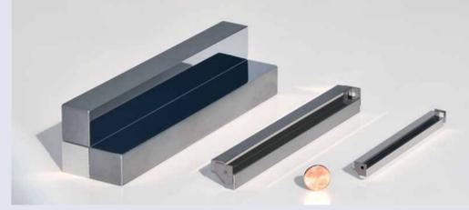
First optics, with slope errors < 2 arcsec, were sold to NSLS and Diamond for scattering experiments.
