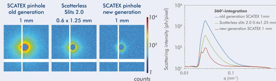
Images of the parasitic aperture scattering at 8 keV with the test apertures being the beam defining element. No scatter guard inserted. The downstream photon flux was the same (variation  $< 1\%$ ) for all compared test apertures.
