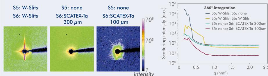
Detector images of the parasitic aperture scattering at 13 keV. In the standard beamline setup S5 denotes the position of the beam defining aperture and S6 the position of the antiscatter aperture.
