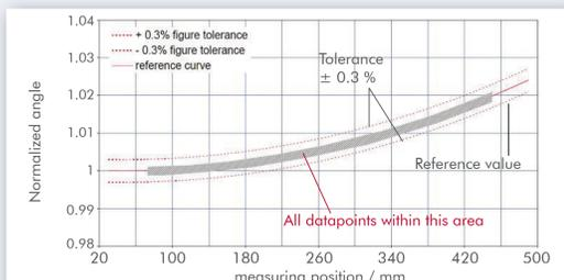
The diagram shows a graded multilayer coating over 500 mm. The deviation of the desired shape in the longitudinal direction is less than  $\pm 0.2\%$ . First optics were sold to the US.
