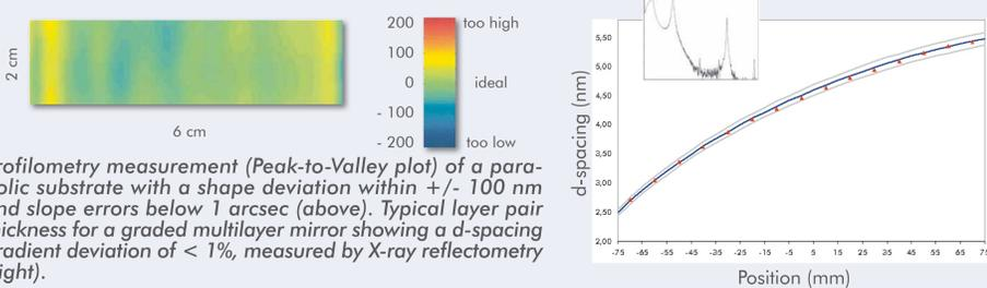
Profilometry measurement (Peak-to-Valley plot) of a parabolic substrate with a shape deviation within  $\pm 100$  nm and slope errors below 1 arcsec (above). Typical layer pair thickness for a graded multilayer mirror showing a  $d$ -spacing gradient deviation of  $< 1\%$ , measured by X-ray reflectometry (right).
