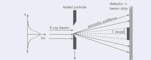
The pinhole is moved stepwise into the X-ray beam while simultaneously measuring the parasitic scattering around the beam stop (above). Scattering patterns and corresponding count rates around the beam stop for 50% of the primary beam intensity passing the pinhole (right).
