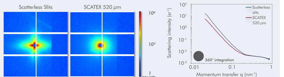
Scattering patterns showing the parasitic aperture scattering at 8 keV for scatterless Ge slits and for a SCATEX pinhole made of Ge (M. Krumrey, C. Gollwitzer, PTB at BESSY II, Berlin).
