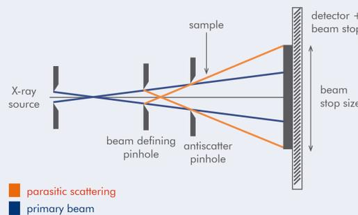
A typical SAXS setup with a 3-pinhole collimation system. Due to the parasitic scattering the beamstop needs to be large in diameter, even with an anticatter pinhole close to the sample. Using SCATEX pinholes, the anticatter pinhole becomes dispensable and the beamstop only needs to have the size of the primary beam uncovering more low resolution data. Further, the beam defining pinhole can be placed closer to the sample.
