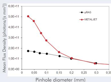
Flux density measurement of the METALJET equipped with a dedicated HELIOS MX optic for protein crystallography. The comparison with a microfocus rotating anode shows that the METALJET is the X-ray source of choice for small and poorly diffracting samples with a size of 0.15 mm or smaller.
