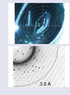
Bruker D8 VENTURE equipped with an IμS<sup>High Brilliance</sup> and an automated ISX stage for in-situ crystal screening and data collection in crystallisation plates at RT; typical diffraction pattern of a Thaumatin crystal.
