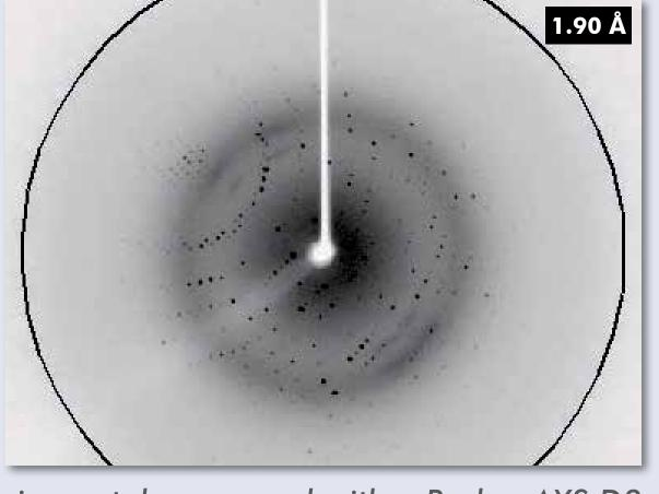
Data statistics and typical diffraction pattern of a small protein crystal, measured with a Bruker AXS D8 VENTURE equipped with the Excillum METALJET X-ray source.
