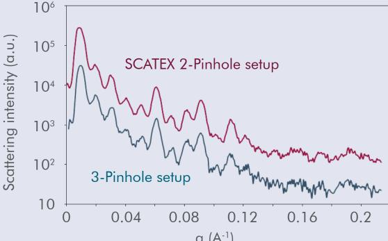
Scattering intensity vs. q-plot, measured with a 3-pinhole high resolution NANOSTAR and a modified 2-pinhole NANOSTAR equipped with SCATEX pinholes. With a similar resolution the SCATEX setup gives a considerably higher scattering intensity.
