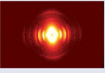
SAXS Image of a thin fiber of a rat tail tendon, measured on a Bruker NANOSTAR with an IµS.
