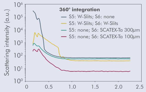
Images of the parasitic aperture scattering at 13 keV. In the standard beamline setup S5 denotes the position of the beam defining aperture and S6 the position of the antiscatter aperture.
