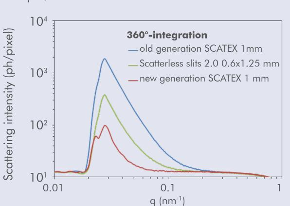
Images of the parasitic aperture scattering at 8 keV with the test apertures being the beam defining element. No scatter guard inserted. The downstream photon flux was the same (variation < 1%) for all compared test apertures.
