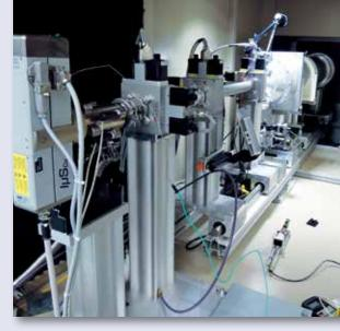
IμS Upgrad on a mar-research 345 dtb a HRXRD setup at Switzerland)
