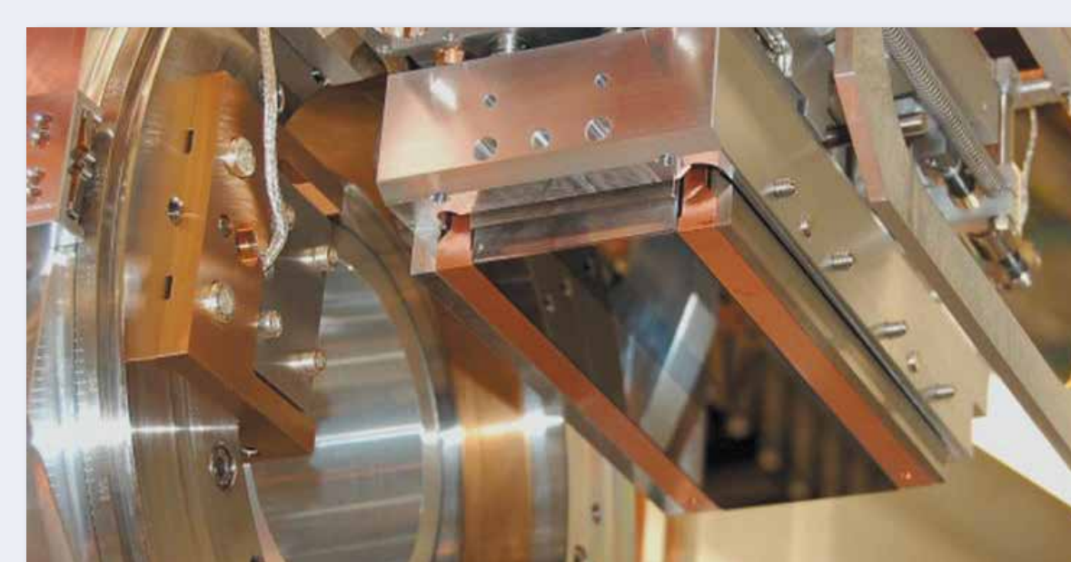
Three-stripe multilayer optics for tomographic microscopy and coherent radiology (TOMCAT at SLS; M. Stapanoni, PSI).
